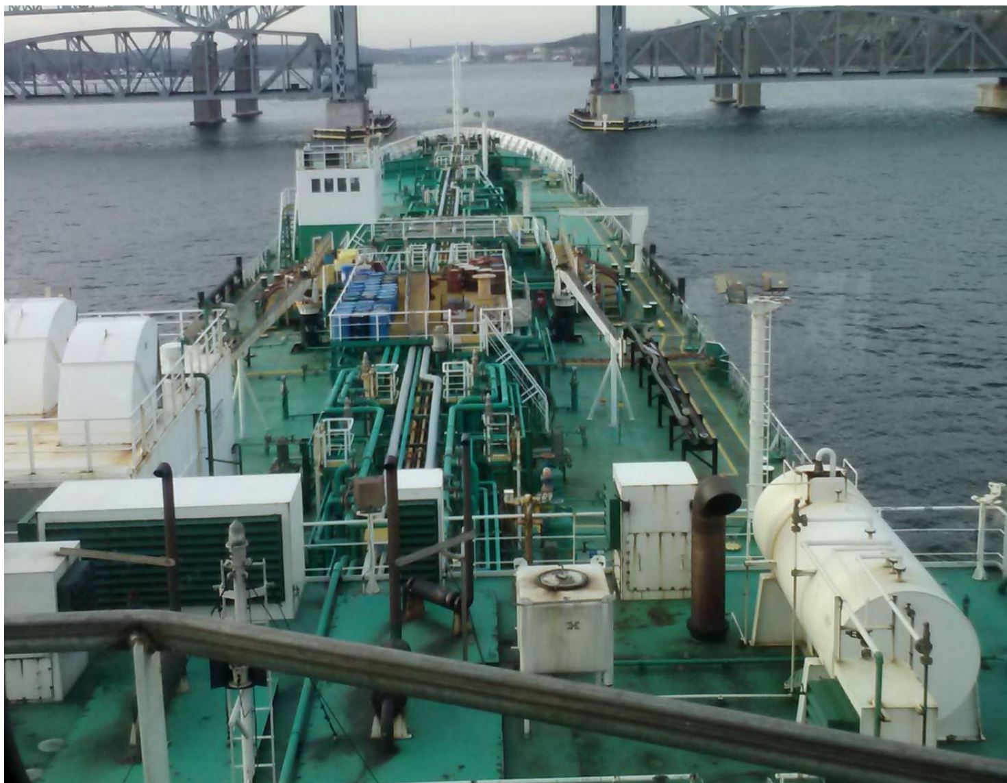
ATB Freeport approaching the Thames River RR Bridge en route to Dow Chemical, Allyn Pt with a cargo of Styrene - Length over all 604 ft, beam 76 ft, Gross tonnage 12,270 Photo - Captain Charles Jonas, Connecticut Marine Pilot
